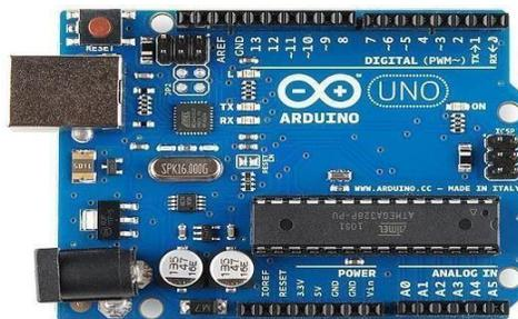
Figure 4.1 – Arduino UNO board
